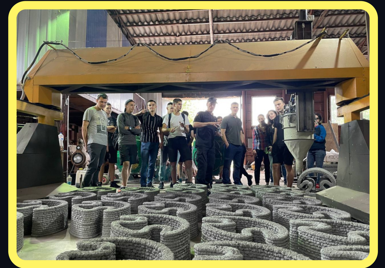
We print structural solutions in the KNUBA laboratory on a construction 3D printer
