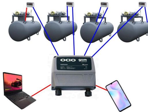
Fig. 1: Fuel level control system
