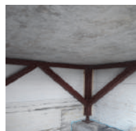
Fig. 2– Installation for tests of structurally - anisotropic plate.
