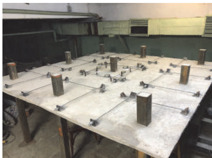
Fig.1 - General view of the reinforced concrete slab reinforced with external prestressed reinforcement
