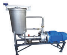
Fig. 2. - Laboratory rotary hydrodynamic homogenizer
