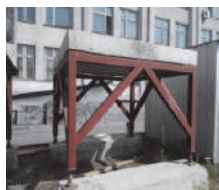
Fig. 2– Installation for tests of structurally - anisotropic plate.
