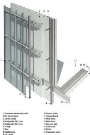
DOUBLE FACADE ISOMETRIC DETAIL
