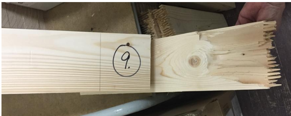
Fig. 1. Failure of a structural glulam beam specimen with a knot defect [6]
