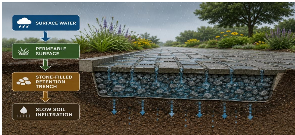
Fig. 3. Retention trenches structure
