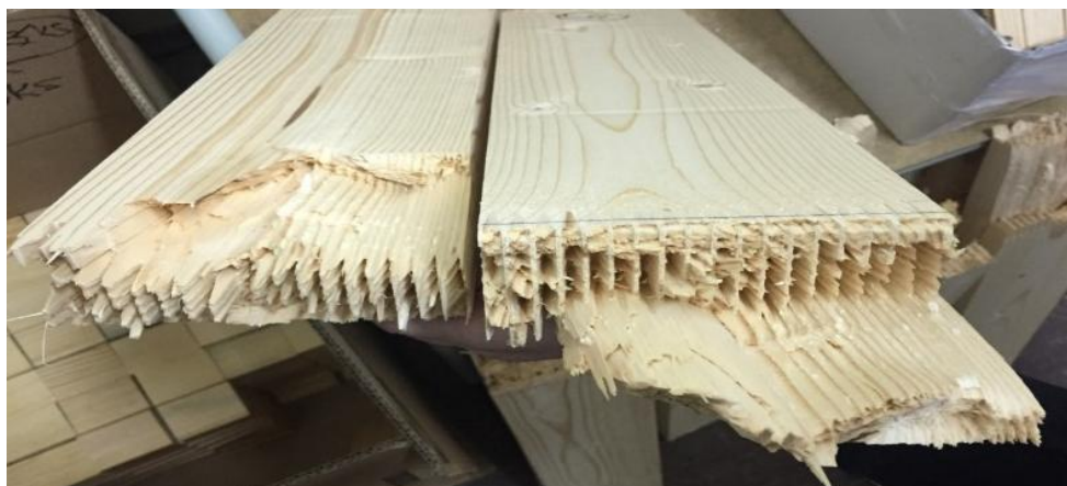
Fig. 2. Failure of a structural glulam beam specimen with a pith defect [6].
